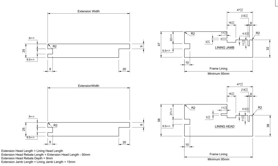
Extension Architrave Head Length = Lining Architrave Head Length Extension Architrave Jamb Length = Lining Architrave Jamb Length
